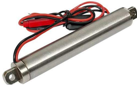
The SL-LA-16 is a compact yet powerful electric linear actuator, engineered to provide impressive performance in a miniature form factor. With a diameter of just 16mm, it delivers a maximum push force of 200N. The actuator features a stainless steel inner and outer tube, providing exceptional durability, while the two end are made from copper alloy for added strength and reliability.
