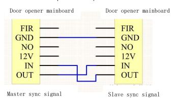
6. Photoelectric beam switch interface, connect to infrared photoelectric beam switch (please use NPN normally open type)
