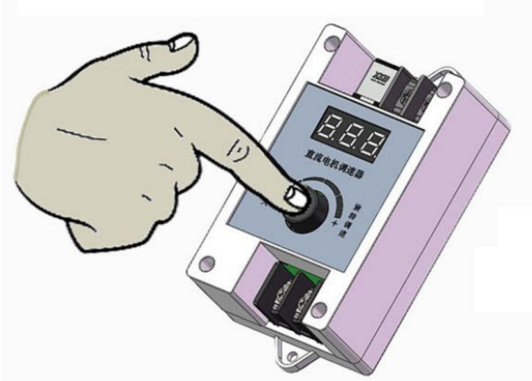
Step 3: L duty ratio off-line setting, range 1%-99%
